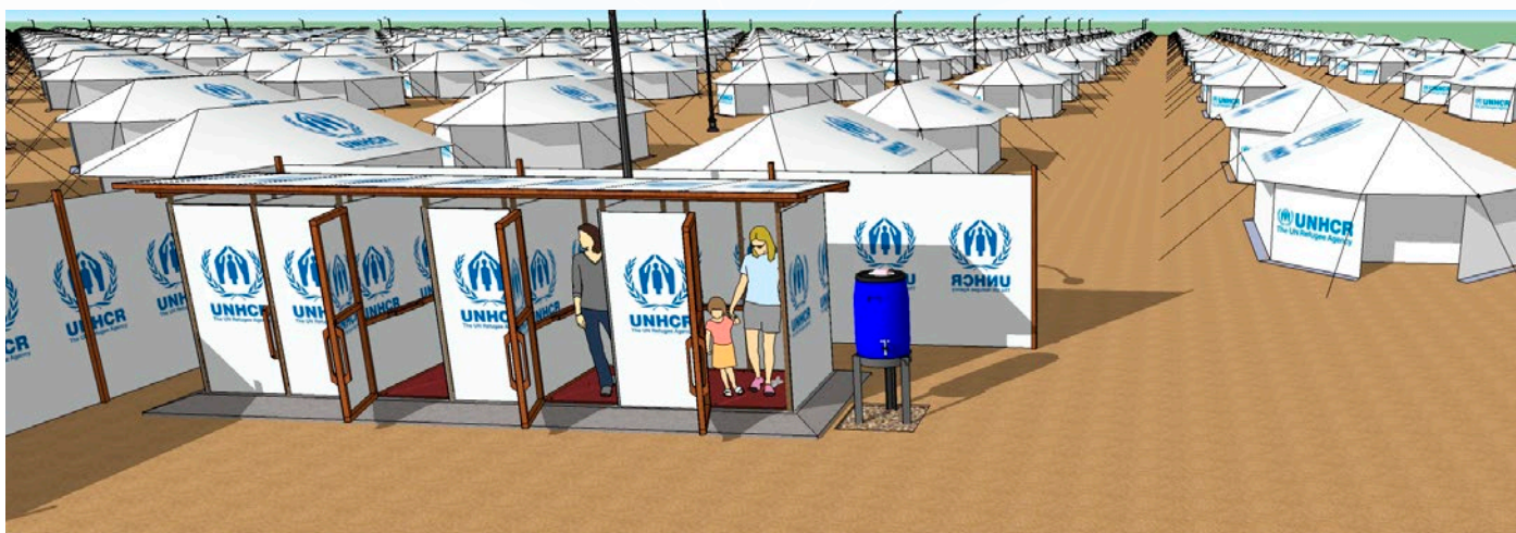
D400-2015a Emergency Trench Latrine Design Poles and Plastic (UNHCR, 2015)
